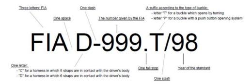
In addition, the labels vary according to the belt on which they are mounted and can be of the following types:
